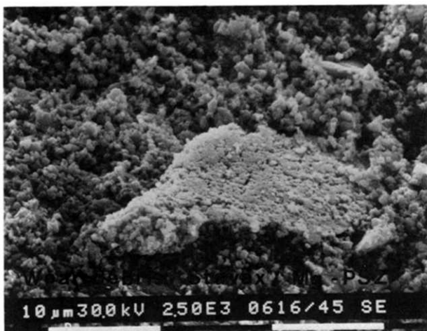
Fig. 10. Wear debris, Mg-PSZ and steel. The figure shows a sheet, containing Mg-PSZ on the visible surface (determined with EDAX) surrounded by oxidized steel spheres.
